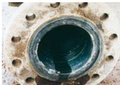
Removal of solidified bauxite from pipes upper: prior to cleaning lower: after cleaning
