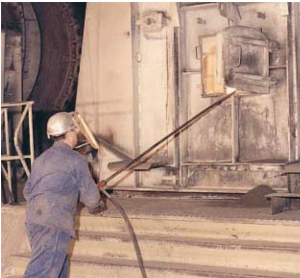
Removal of accretion rings in rotating kilns by water jet lances
