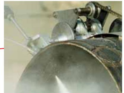
On-site pipe cutting with the 3000-bar abrasive system Eco Top Cutter 3000.
