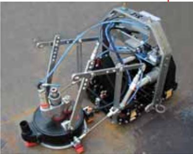
The Magnetic Lizard M2500 is a self-propelled cleaning system which is adhered onto the surface via permanent magnet.
