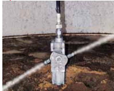
Internal vessel and tank cleaning with the tank cleaning head TankMaster® and the corresponding positioning device.
