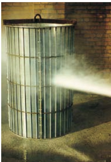
Filter cleaning using a high-pressure water jet
