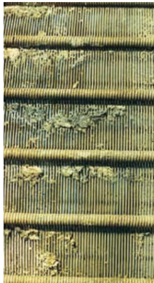
Cleaning results on a filter cleaned by high-pressure water jetting
