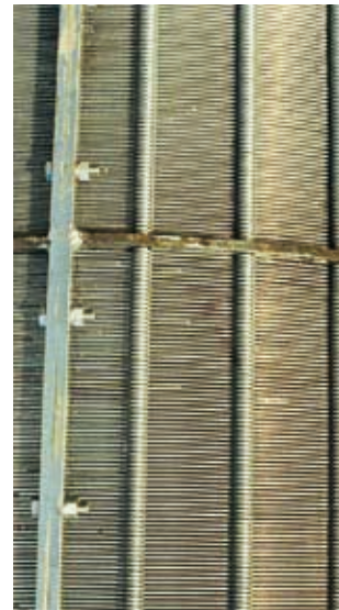
Cleaning results on a filter cleaned by high-pressure water jetting
