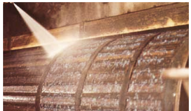
Cleaning of sieve-suction-rollers with high-pressure water lances
